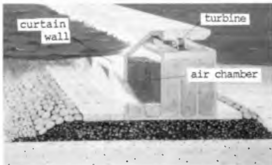
Fig.1 Wave Power Extracting Caisson Breakwater
