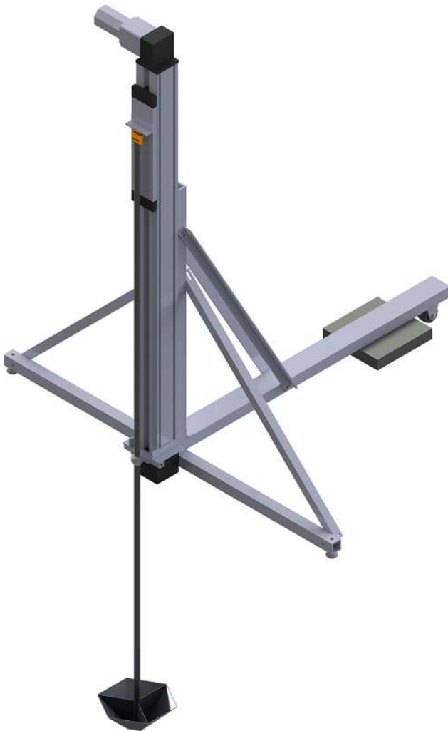
Fig. 1. Oscillator test apparatus, which is mounted to the edge of a dock and uses a linear actuator to force submerged heave plate oscillations with a pushrod.
