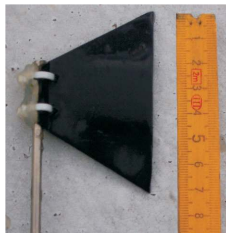
Fig. 2. Artificial fin used for generation of hydrodynamic trails.
