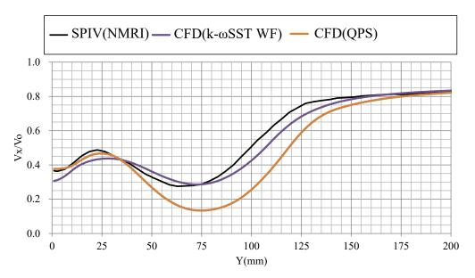
**Figure 10.** Longitudinal velocity distribution along the horizontal line above the propeller shaft calculated by wall function models.
