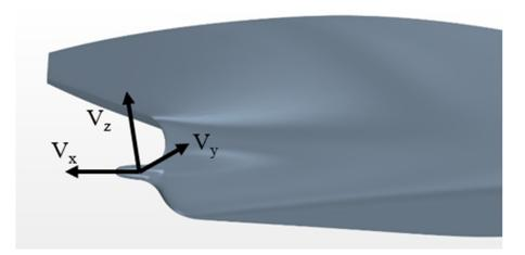
Figure 6. Coordinate system of the CFD calculation.
