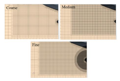
**Figure 5.** Grid arrangement around the propeller plane.
