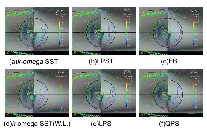
**Figure 8.** Crossflow distribution of SPIV (Left) and CFD (Right) at 110 mm from AP to bow side. (a) *k*-omega SST (b) LPST (c) EB (d) *k*-omega SST (W.L.) (e) LPS (f) QPS.
