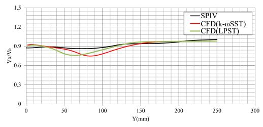
Figure 19. Axial velocity distribution of Model5415 along the horizontal line above propeller shaft.
