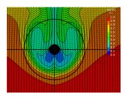
**Figure 14.** Comparison of results of the wake distribution of KVLCC2. ((**Left**): EFD, (**Center**): *k*-omega SST, (**Right**): LPST).
