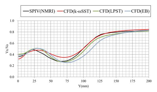
**Figure 11.** Longitudinal velocity distribution along the horizontal line above the propeller shaft calculated by low Reynolds number models.
