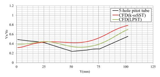
Figure 17. Axial velocity distribution of KVLCC2 along the horizontal line above propeller shaft.
