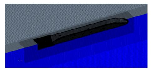
**Figure 3.** Volume grid of JBC around the hull.
