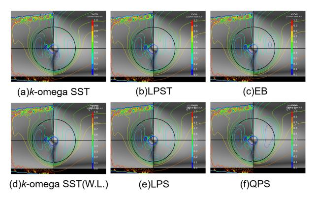
**Figure 7.** Distribution of longitudinal velocity of SPIV (Left) and CFD (Right) at 110 mm from AP to bow side. (a) *k*-omega SST (b) LPST (c) EB (d) *k*-omega SST (W.L.) (e) LPS (f) QPS.
