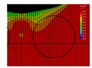
**Figure 16.** Comparison of results of the wake distribution of Model5415. ((**Left**): EFD, (**Center**): *k*-omega SST, (**Right**): LPST).
