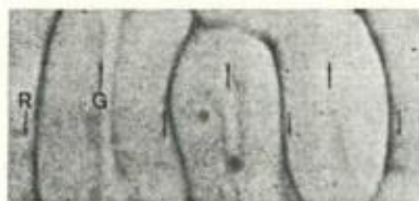
Fig. 3 Surface patterns showing convective movements in an aqueous solution of chromogenic developer during irradiation. ↓, Down; ↑, up; R, red; G, green.
