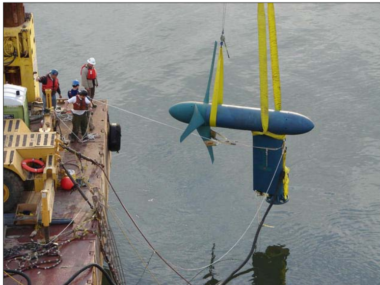
Figure 1. The Verdant Power 35-kW hydrokinetic turbine
