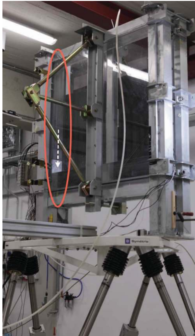
FIG. 3. View of the plexiglas tank reinforced with aluminium and steel structures. The red oval highlights the left lateral wall built in stainless steel and holding the deformable aluminium plate (indicated by the white arrow).
