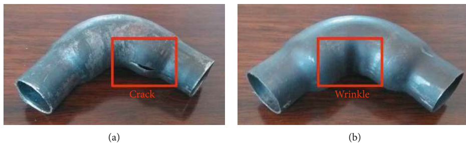
FIGURE 5: Defections in the forming process: (a) crack and (b) wrinkle.
