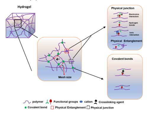
Figure 4. The structure of hydrogels (chemical linking and physical junctions).
