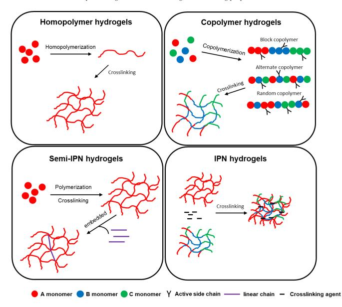
**Figure 3.** Simple diagram of homopolymer hydrogels, copolymer hydrogels, semi-IPNs, and IPN hydrogels.
