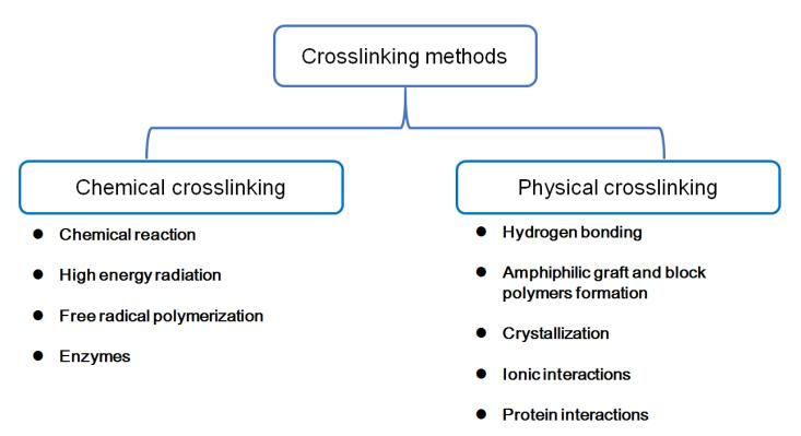
Figure 5. Methods of chemical and physical crosslinking for hydrogels preparation.
