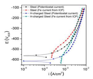
Figure 7. Influence of hydrogen charging on 1018 steel [61].
