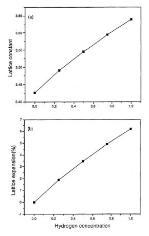
Figure 6. Lattice constant (a) lattice expansion (b) changes with concentration of Hydrogen [60].
