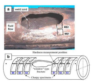
Figure 5. (a) damaged boiler tube facture; (b) position of facture on the boiler tube [56].
