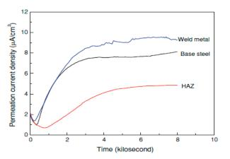
Figure 9. Hydrogen permeation current curves [73].
