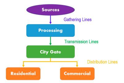
Figure 4. Natural gas pipeline network diagram.
