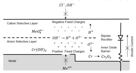
Figure 8. Schematic: bipolar passive film model (adapted from [72]).
