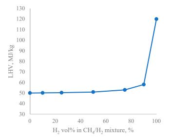
Figure 3. LHV of methane-hydrogen mixtures (Data from references [15,16]).
