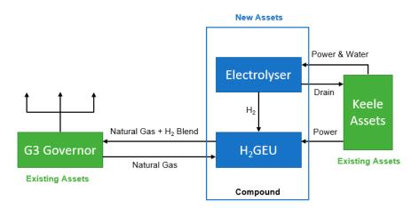
Figure 11. HyDeploy process design flow chart (adapted from [76]).
