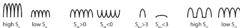
Figure 3.6 Illustration of a selection of important surface topography and functional parameters ( S_a , S_{sk} , S_{ku} , and S_{ci} ) that were assessed by profilometry.
