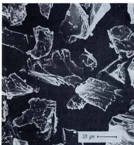
Fig. 2 — Scanning electron micrographs of \text{LaNi}_5 after a few hydrogen absorption/desorption cycles.
