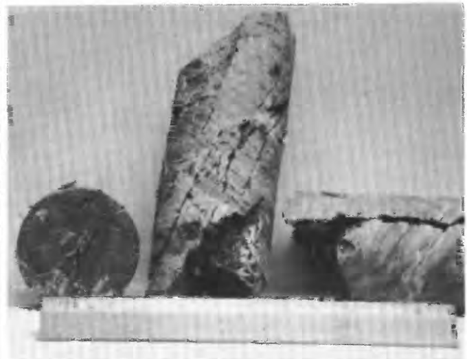
FIGURE 7. — Sealed, vuggy, and open fractures in cores of carbonate rock from the Pogonip Group, well 88-66, Yucca Flat. Cores are from depths of 2,705 to 2,787 feet below surface.
