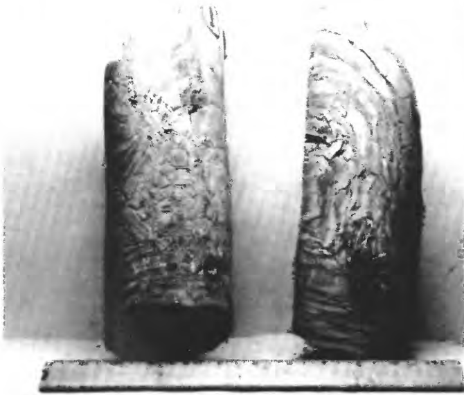
FIGURE 6. — Structure in cores of Pogonip Group, well 88-66, Yucca Flat. Left core (depth 2,980 ft), folded limestone (light gray) and shale (medium gray). Right core (depth 2,983 ft), fault breccia of limestone fragments. In both cores the fragmented limestone is tightly cemented by clayey or shaly gouge.
