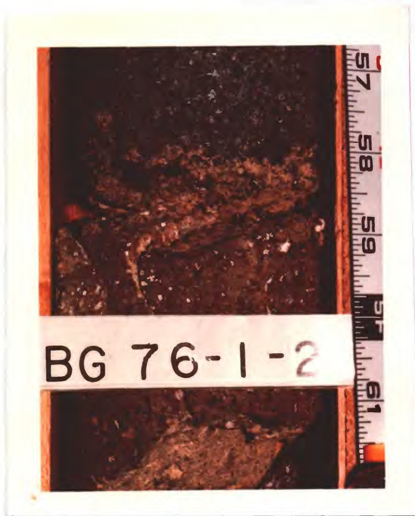
Figure 8.--Photograph of mineral deposits in vesicles immediately below a basalt flow contact in well 76-1, at a depth of 28.13 meters.
