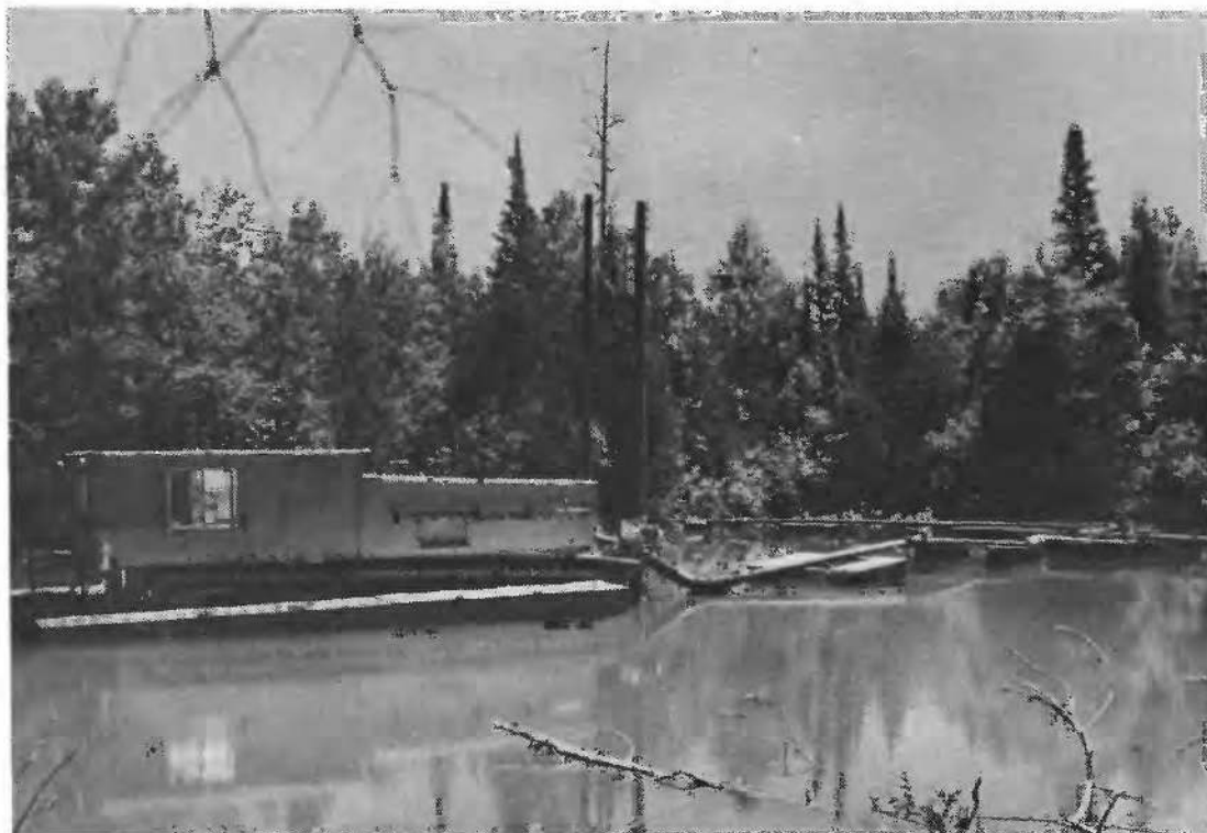
Figure 9. Hydraulic dredge in operation at Sunshine Pond.
