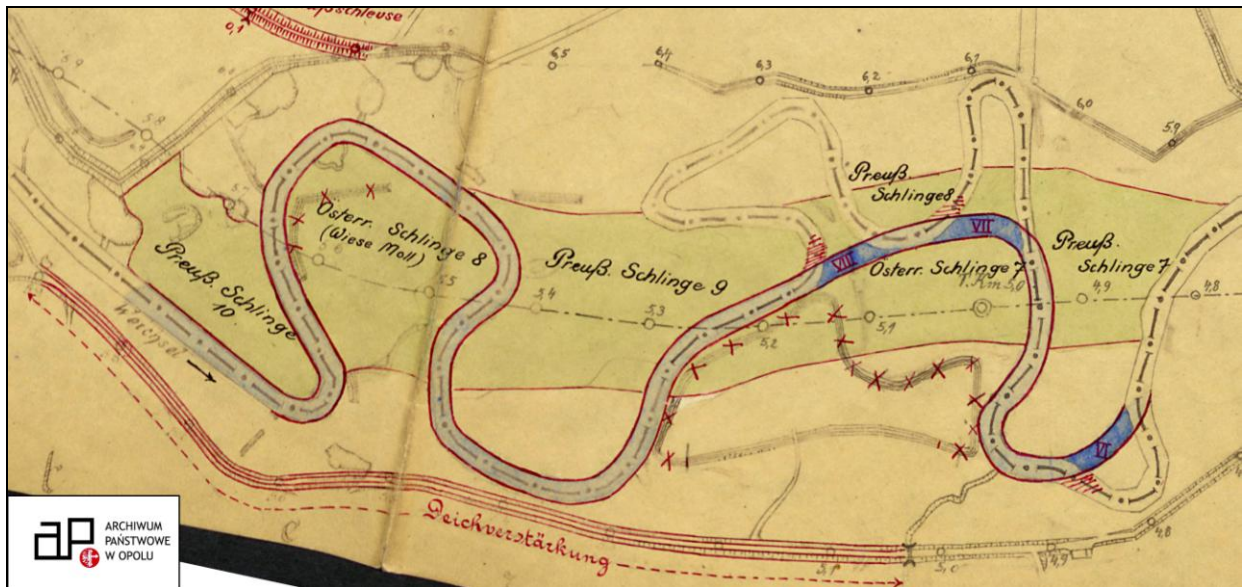
Fig. 9. River engineering work design – River Vistula valley (after Regulierung der Österreichische Weichselstrecke, 1892–1901, original scale: 1:5000, State Archives in Opole)
