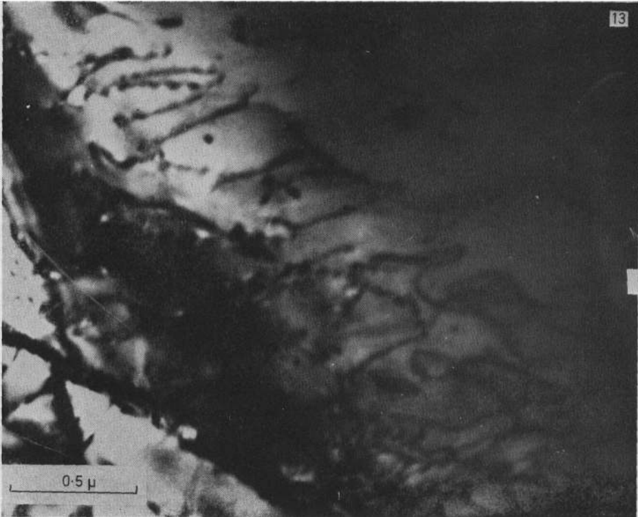
FIG. 13. Synthetic quartz crystal deformed under conditions of hydrolytic weakening. Dislocation lines curved and tangled in contrast to Fig. 12.
