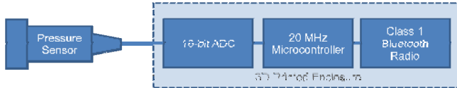
Figure 4: Our prototype sensor implementation. The sensor twists on to a fixture and communicates wirelessly.
