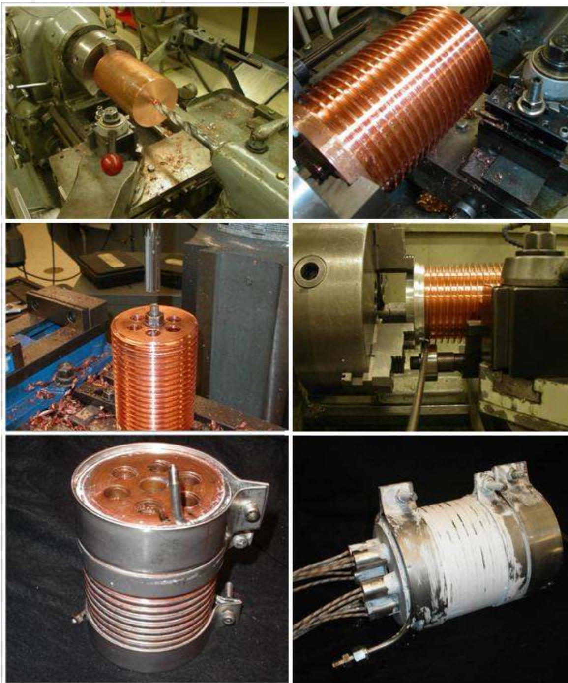
Figure 7.8 Photographs of preheater construction process. From upper left: drilling center hole; grooving thread; drilling and reaming heating element holes; wrapping high pressure tubing around block into threads; block with tubing wrapped and secured with clamps; finished preheater with heating elements inserted.
