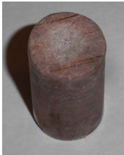
Figure 8.12 Sioux quartzite successfully spalled using 15 mass% methanol fuel flame jet.
