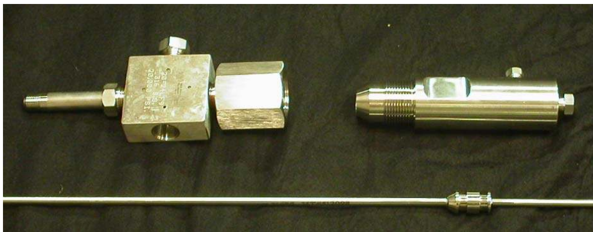
Figure 7.11 Photograph of movable probe assembly. Clockwise from upper right are HIP fittings (nipple, tee, and adapter, assembled), cylindrical housing, and tubing with piston welded in place.
