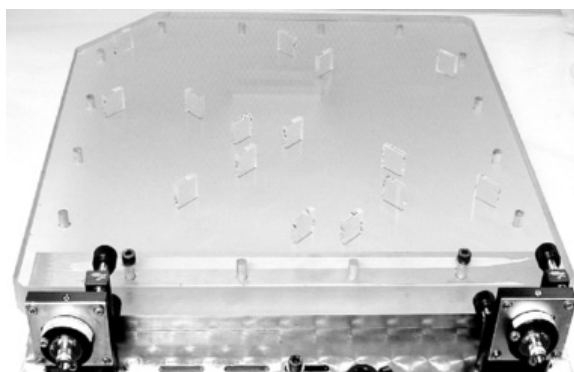
Figure 5. Prototype optical bench fabricated using hydroxide-catalysis bonding.
