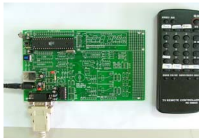
Fig. 6. The IR receiver and the remote controller
