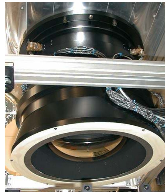
Wide field corrector developed by Canon
