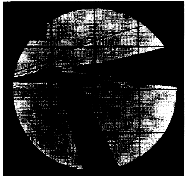
Figure 16 (b). Schlieren photograph from AEDC Tunnel B Mach 6 separation tests for A_{sep} = 0^\circ , x_{sep} = -20^\circ .
