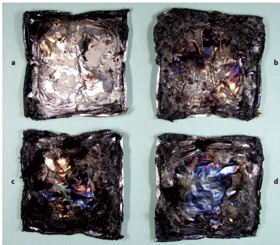
Figure 7. Cone calorimeter residues of a) EP, b) EP + PDTT, c) EP + DOPO-HQ, and d) EP + OPPh 3 .
