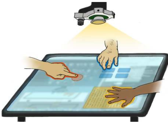
Figure 6. Concept sketch showing use of HyperCam to identify users on a multi-touch tabletop display
