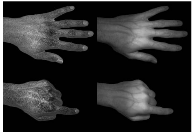
Figure 7. Hand images captured by HyperCam that accentuate either hand texture ( Left ) or venous structure ( Right )
