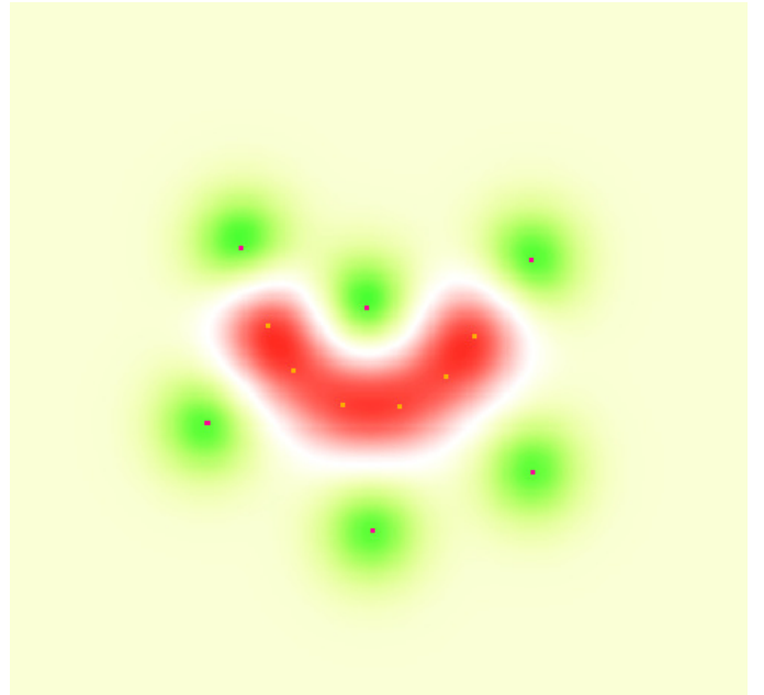
Fig. 8. For very local kernels, the decision function of the SVM can be close to 0 (light color in this picture) for a large part of the input space, so very many items can be mapped to the vicinity of the discrimination hyperplane in feature space.
