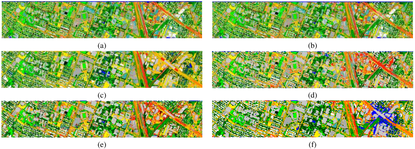
Fig. 8. Classification maps for Houston data: The outputs of RF on (a) hyperspectral data, (b) the stack of LiDAR and hyperspectral data, and (c) the proposed approach using feature stacking; the outputs of CNN-based classification on (d) hyperspectral data, (e) the stack of LiDAR and hyperspectral data, and (f) the proposed approach using GBFF.
