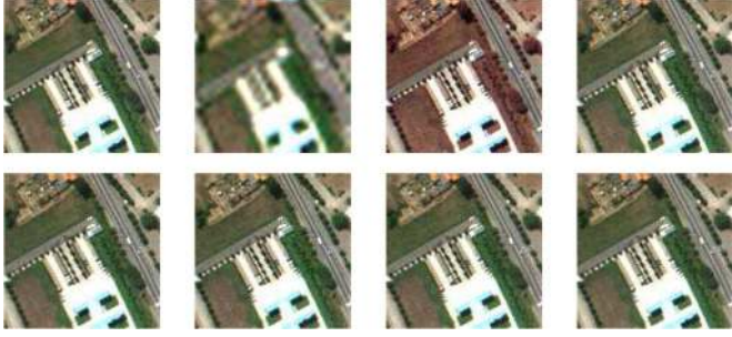
Fig. 6. Pavia data set. (Top 1) Reference. (Top 2) HS. (Top 3) MS. (Top 4) MAP [14]. (Bottom 1) Wavelet MAP [17]. (Bottom 2) Coupled nonnegative matrix factorization (CNMF) fusion [18]. (Bottom 3) MMSE estimator [16]. (Bottom 4) Proposed method.
