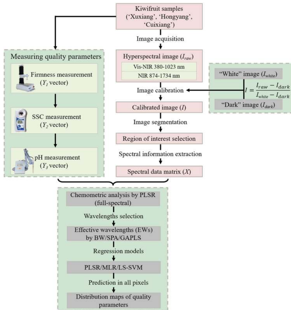
Figure 6. Flowchart of image preprocessing and data analysis for predicting internal quality of kiwifruits.
