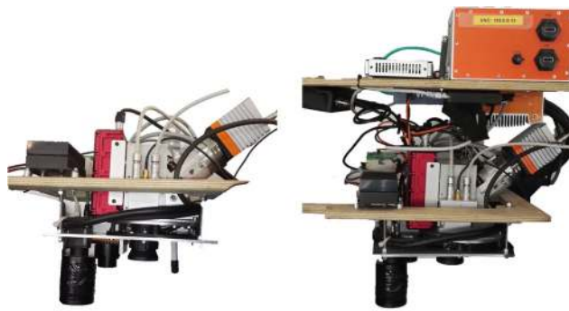
(a) Side view of the payload, (b) Side view of the full pay- with imaging sensors and IMU load. unit.
