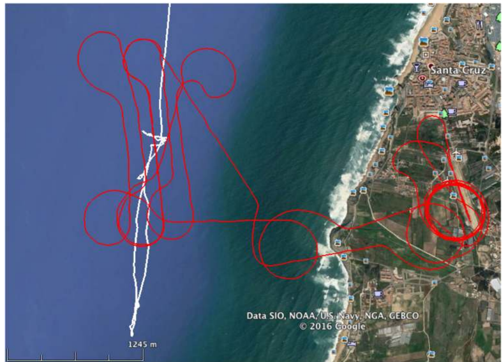
Fig. 12 In red color the ANTEX UAV flight trajectory during the flight, and in white color the boat ground-truth position information
