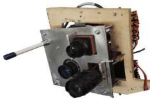
(c) Bottom view of the pay- load, showing all imaging sen- sors and the AIS antenna.
