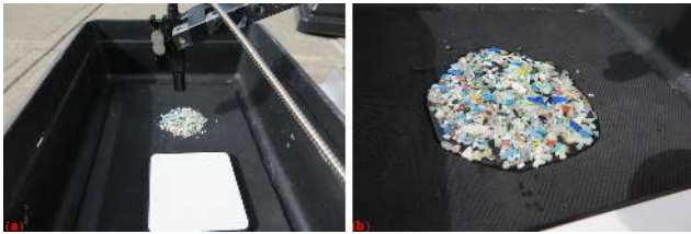
Figure 1. Experimental setup with the aggregated (a) dry and (b) wet marine-harvested microplastics. Black neoprene rubber was used as a background in a dark spray-painted container to mitigate background light during spectral reflectance measurements.
