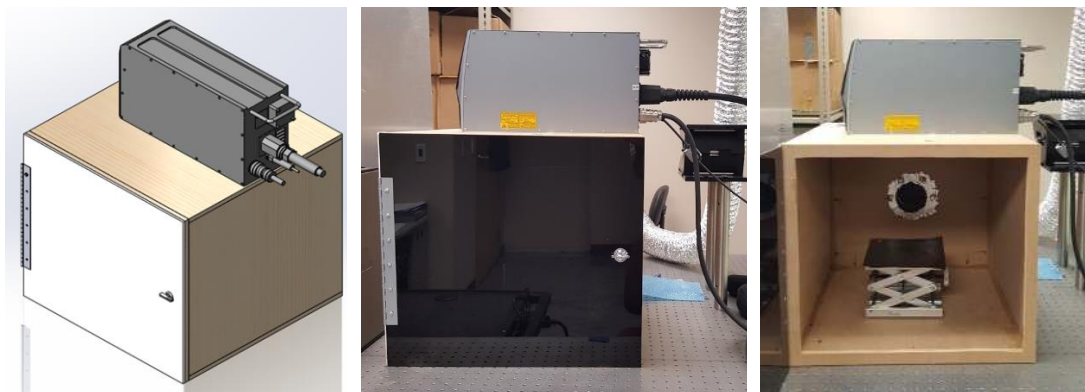
Figure 3.1 (a) CAD Model of laser mounted on the enclosure (b) Keyence Laser mounted on developed enclosure (c) Graphene sheet placed for cutting.
