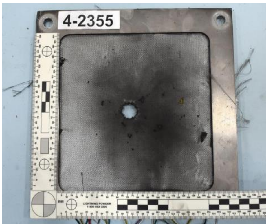
Figure 5.27 Back side of the second layer (inkjet-printed sensors) after the second test
