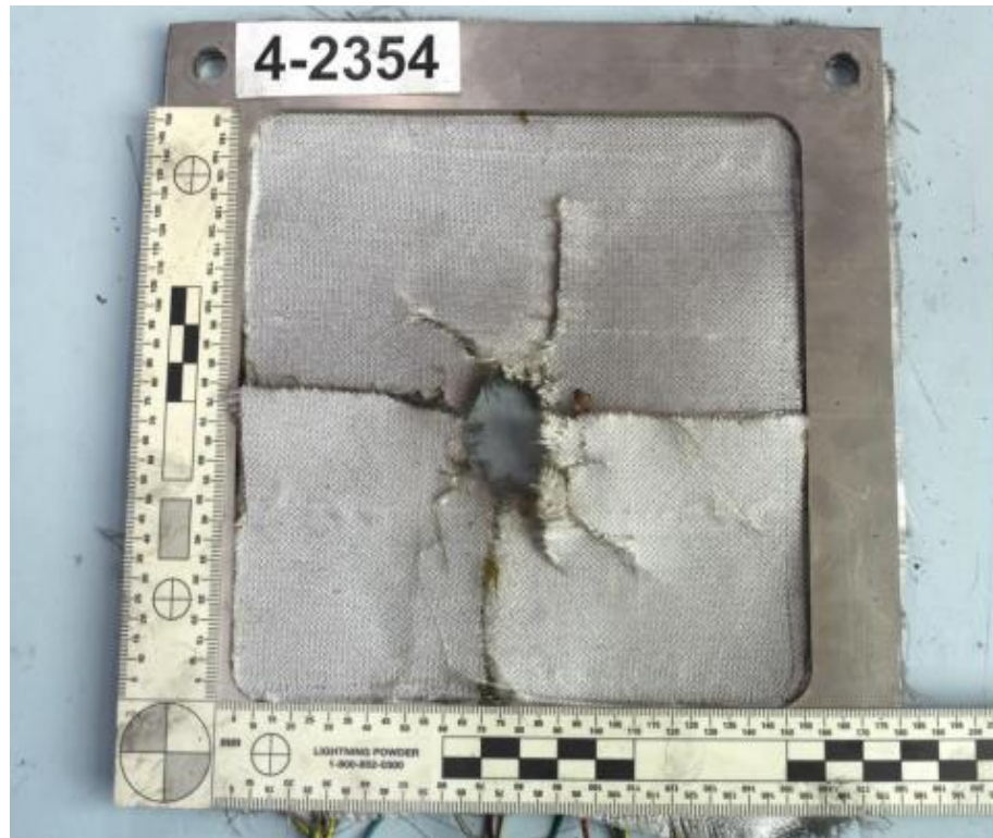
Figure 5.20 Back side of the third layer (ink jet printed sensors) after the first test
