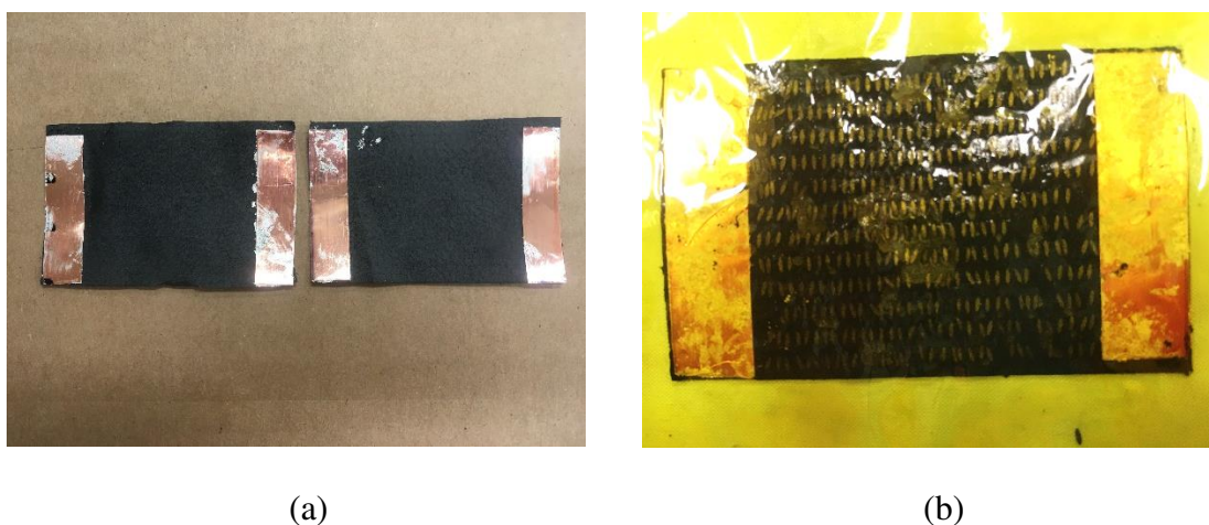
Figure 3.5 (a) CNT sheet with copper electrodes (b) Patterned elliptical GNP-CNT hybrid nanocomposite
