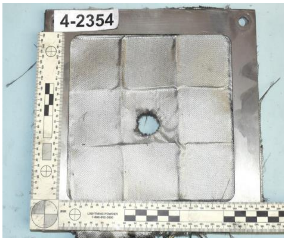
Figure 5.18 Back side of the second layer (hybrid sensors) after first test
