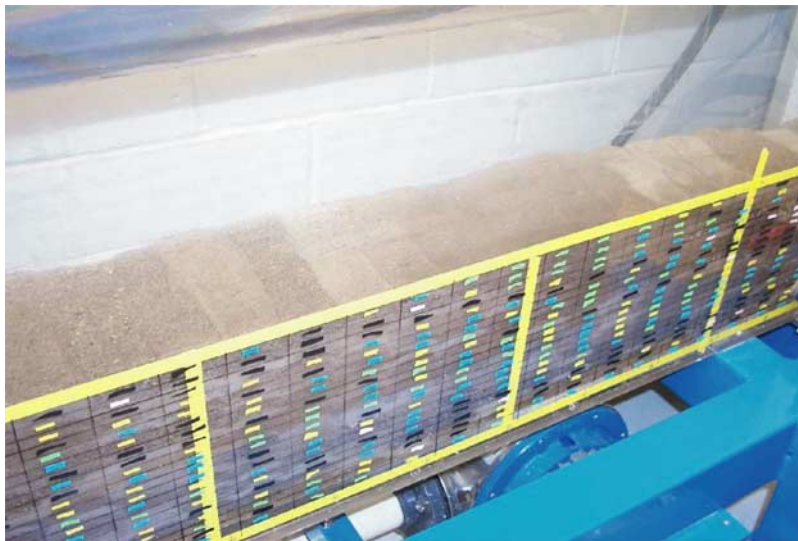
Figure 3. Lower heterogeneity bed in the recirculating flume. The grid on the channel sidewall is color-coded to indicate the sand type in each block.
