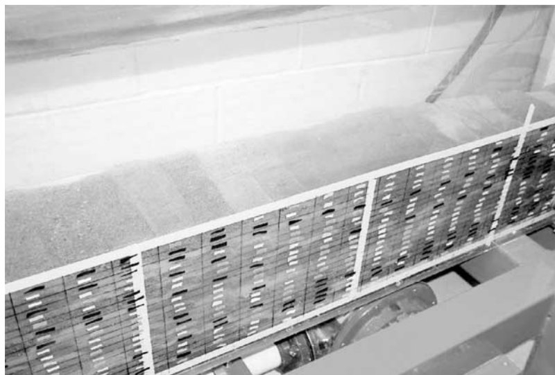
Figure 3. Lower heterogeneity bed in the recirculating flume. The grid on the channel sidewall is color-coded to indicate the sand type in each block. See color version of this figure at back of this issue.
