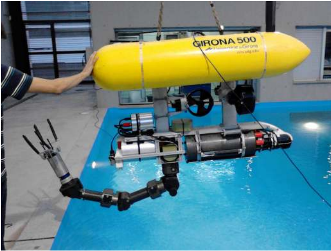
Fig. 4. The I-AUV during the first integration trials at the water tank in the Underwater Robotics Research Center of the University of Girona. The UJIOne gripper can be seen mounted at the end of the UMA. The JR3 sensor is the thin dark band at the wrist of the gripper.
