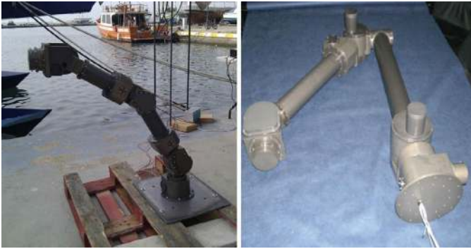
Fig. 3. Different configurations of the arm are possible because of its modular conception. On the left, the arm with 7 DOF, on the right, with 6 DOF.
