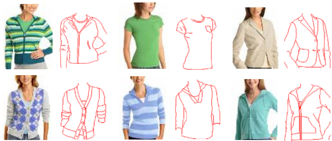
Fig. 18. Sketch graph representation of cloth. The sketch graph can effectively capture internal structural information of cloth, such as folds, sewing lines and albedo/lighting changes.
