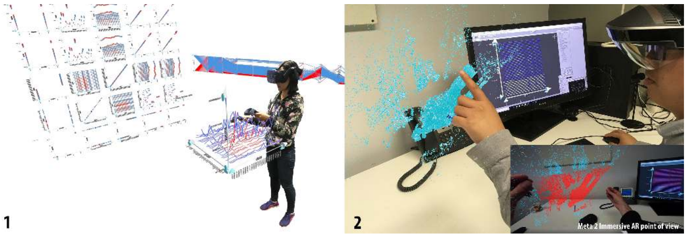
Figure 6: Two examples of immersive visualisation with IATK 1) An immersive VR visualisation platform to analyze multidimensional data (Dow Jones dataset). The user brushes a 3D trendline visualisation and the points are highlighted in red in both the scatterplot matrix and the parallel coordinates. 2) An augmented desktop visualisation platform with the Meta 2. The user interacts with a map displayed in AR above the physical desktop, and the selected data points highlight on the 2D visualisation on screen in Unity.
