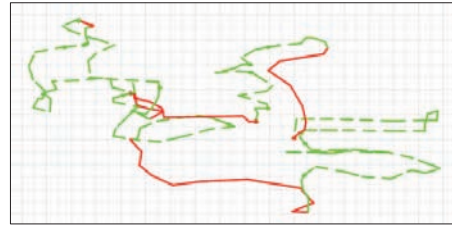
Figure 2. One taxi's GPS trace in two hours, where red (solid) or green (dashed) indicates the taxi is occupied or vacant.
