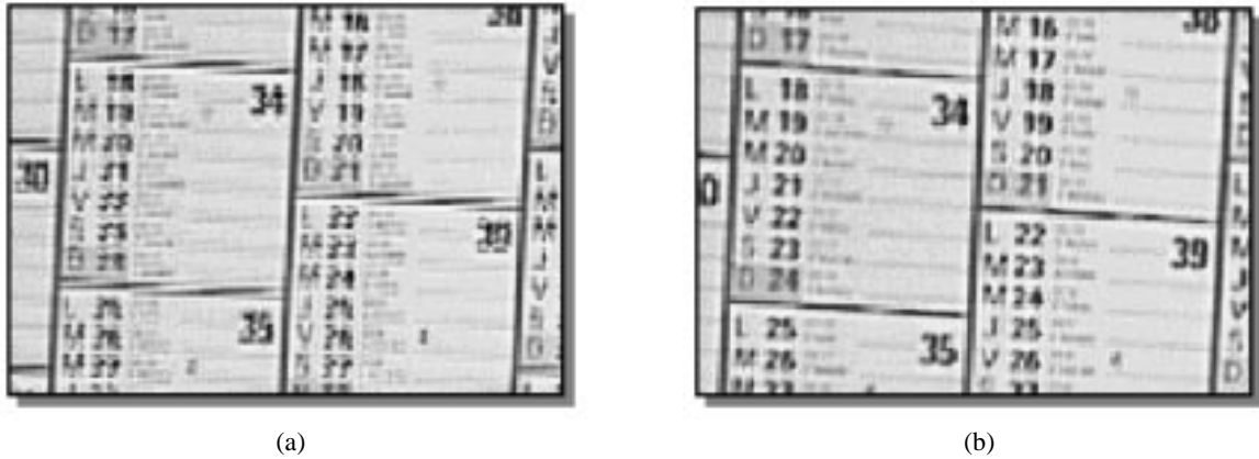
Fig.4 Photographs of a screen detail comparing one of the best non-motion compensated methods, vertical temporal filtering (a) with the de-interlacer in the current IC (b). The pictures are part of a sequence in which the calendar moves upwards with a velocity somewhere between 1 and 2 pixels per field period.
