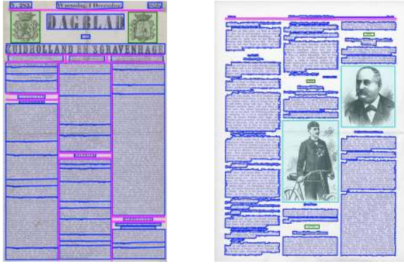
Figure 2. Sample images showing the ground-truth region outlines (blue: text, magenta: separator, green: graphic, cyan: image).
