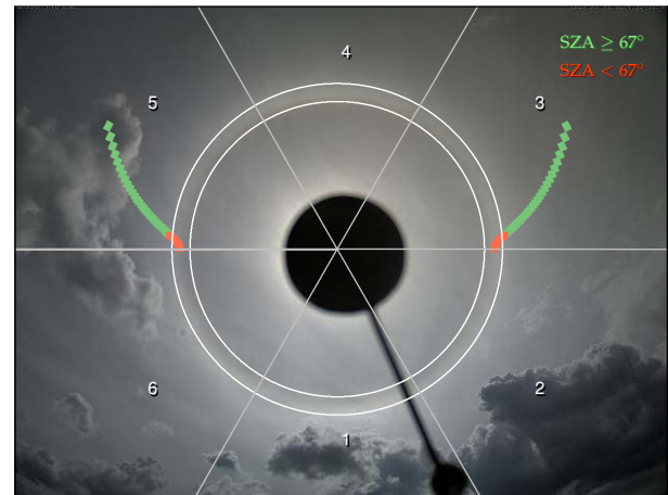
Figure 9. HaloCam image as in Fig. 4b. The red and green squares indicate the minimum scattering angle of the sundogs as a function of the solar zenith angle (SZA). The SZA ranges between 90 and 35° with 1° resolution. The mask used to search for the 22° halo peak is displayed by the two white circles and covers scattering angles between 21.0 and 23.5°. Sundog positions located within this mask might be misclassified as 22° halo and are marked as red. These positions correspond with SZAs between 90 and 67°. For smaller SZAs (higher solar elevations) the sundogs are located outside the mask and cannot be misclassified as 22° halo by the algorithm.
