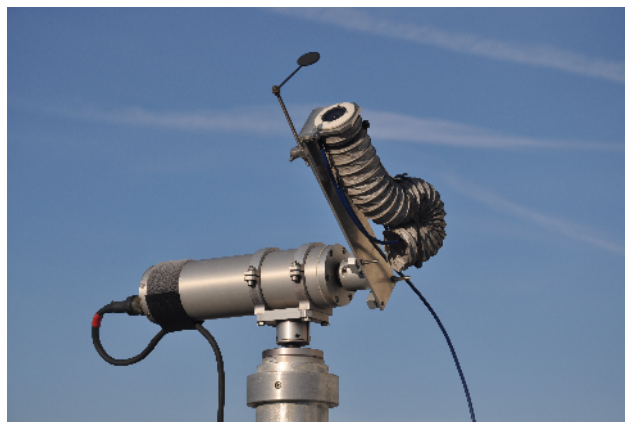
Figure 2. HaloCam: wide-angle camera (Mobotix S14D) with circular shade on a sun-tracking mount. The mount consists of two axes with stepping motors to adjust azimuth and elevation of the camera.
