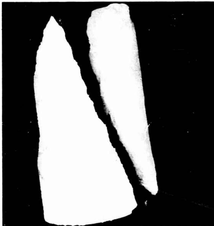
Figure 13. Horizontal, compression specimen tested at -20^{\circ}\text{C} , showing typical shear failure.
