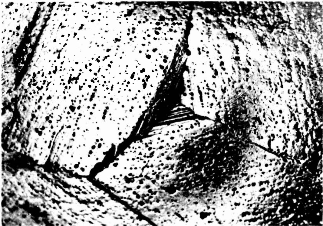
Figure 36. Strain slippage at boundary intersection of three crystals.
