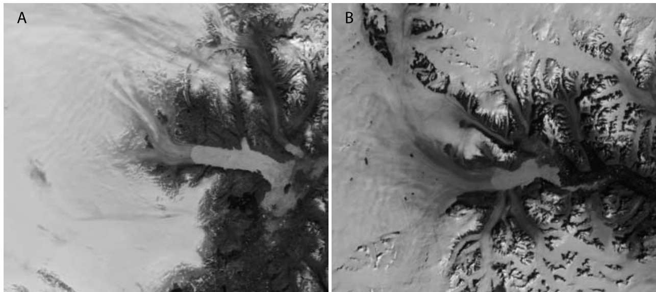
Figure 1. Examples of MODIS images used to determine front positions for (a) Helheim (19 July 2005) and (b) Kangerdlugssuaq (24 August 2005). Note different polar stereographic projections were used so that the glacier flow direction would be aligned approximately with the horizontal direction.
