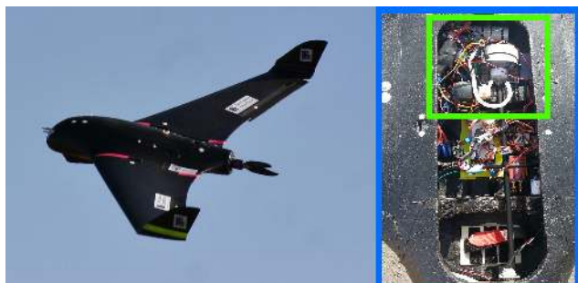
Figure 7. The Skywalker UAS with the single-sample aerosol collector (green rectangle; photograph by Christos Keleshis).
