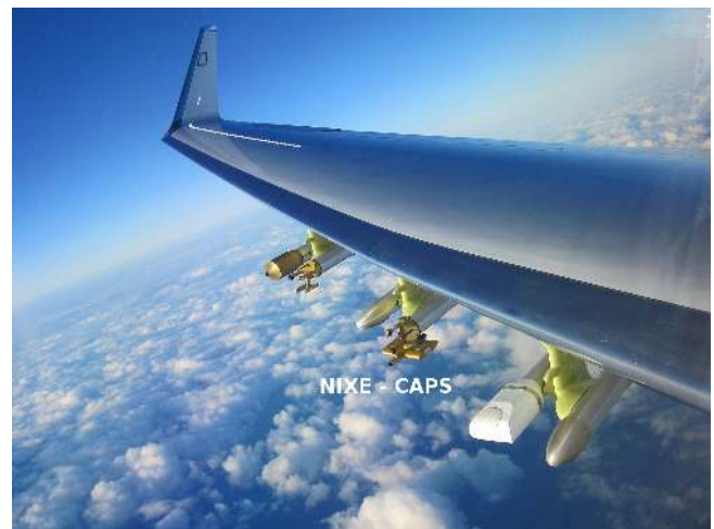
Figure 7. NIXE underwing mounting on HALO (photo: Armin Afchine).
