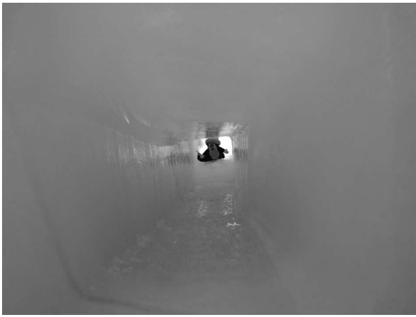
Fig. 7. First channel melted by IceMole 1 at Morteratschgletscher in 2010: 45° upwards, length ~1.5 m.
