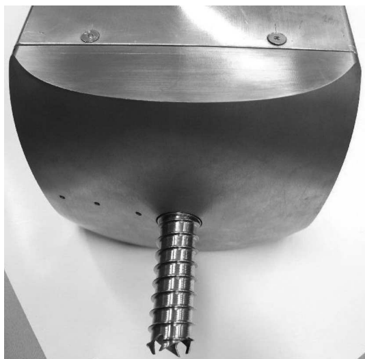
Fig. 3. IceMole 1 melting head with ice screw.
