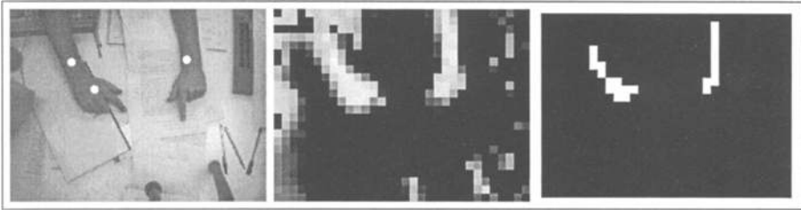
Fig. 2. Colour segmentation allows the detection of skin-coloured blobs. Circles on the input frame (left) show the centres of blobs detected using colour-segmentation and a flood-fill. The output of the colour discriminant on a 32 \times 24 pixel subsampled field of the original image is shown scaled (middle) so that white corresponds to a high probability of skin-colour. The output after convolution and blob-detection (right) shows white areas belonging to blobs.
