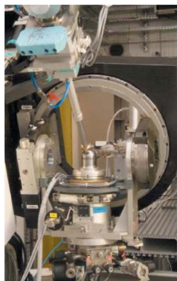
Figure 3 Left: azimuthal set-up mounted on the \Phi circle of the MicroControle diffractometer. Right: drawing of the azimuth sample rotation stage which allows the full rotation of the Displex around its axis \rho . \psi is the azimuthal angle around the scattering vector \mathbf{Q} . The incident light polarization \epsilon_r is perpendicular to the vertical scattering plane defined by the incident and scattered photon wavevectors \mathbf{k} and \mathbf{k}' , respectively.
