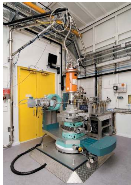
Figure 4 General view of the experimental hutch EH2 with the ^4\text{He} evaporation cryostat mounted on the Huber six-circle diffractometer.
