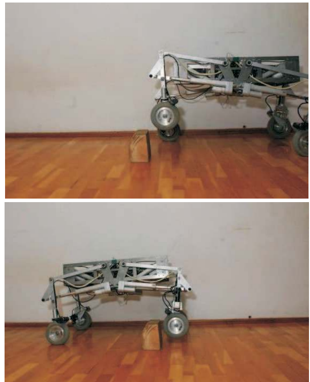
Fig. 7. Obstacle negotiating function – obstacle in front of one limb
