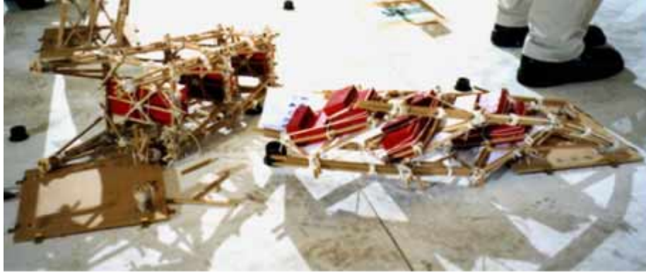
Figure 8: Typical failures observed during the shaking table testing.
