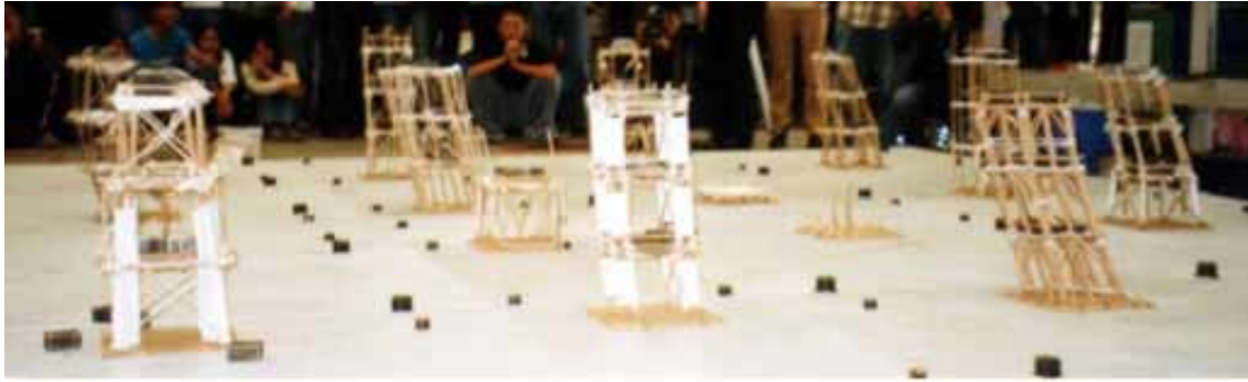
Figure 8: Some of the Taiwanese models being tested on the NCREE shaking table. Note the large sway deflections in several of the softer models.
