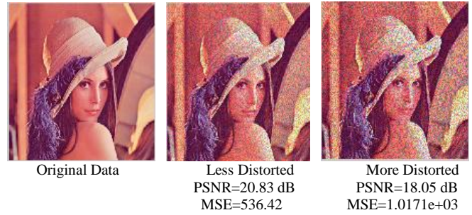
Fig. 3 PSNR calculation of various images
